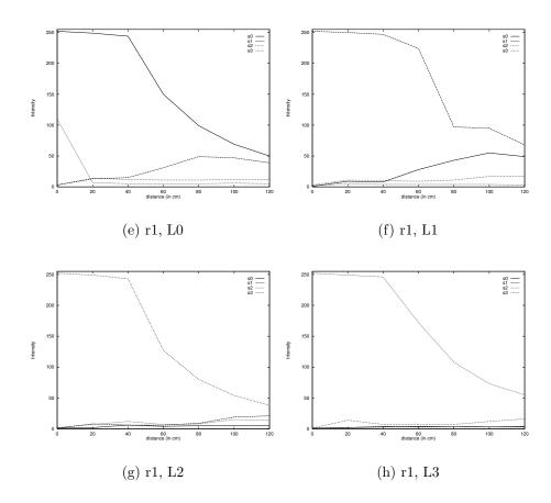
Figure 2.5: The characteristics of the calibrated light sensors as empirically measured for the experimental set-up when exposed to light sources L0 - L3. Plots (a) - (d) show the of robot r0 and plots (e) - (h) show them for r1. The distances are measured from the front of the robots to the boxes. Actual distances from source to sensor are 12cm further.
