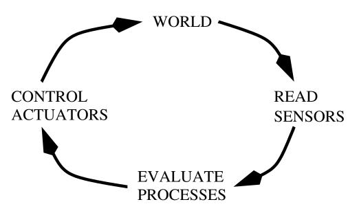
**Figure 2.7:** The way that PDL interacts with the world via a robot. Every  $\frac{1}{40}s$  PDL is going through a cycle as shown in the figure.
