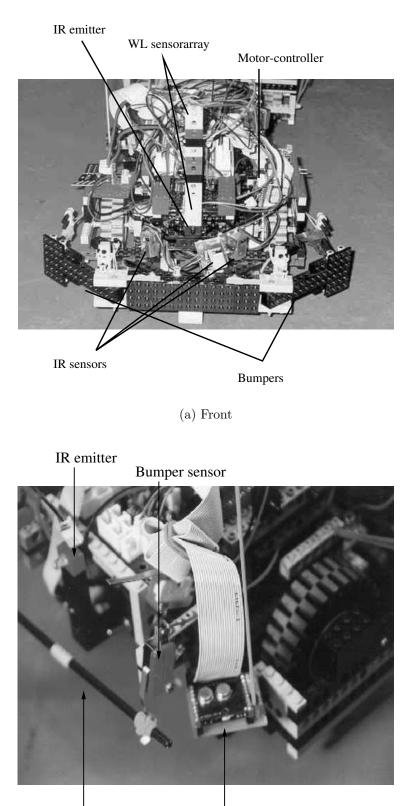
Radio-link module Bumper construction
