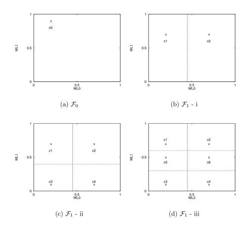
**Figure 3.7:** These figures show feature spaces  $\mathcal{F}_0$  (a) and  $\mathcal{F}_1$  (b), (c) and (d), each with their prototypes (x) as used in the example. The figures are displayed in two dimensions for illustrative purposes; in the actual implementation the spaces have 4 dimensions.
