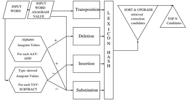
Figure 1: The core-correction mechanism. The lexicon built up from the input word list is queried for transpositions on the basis of the Input word Anagram Value (IAV) alone. Each AAV is added to the IAV to query for deletions. Each TAV is subtracted to query for insertions. Each AAV is added and each TAV subtracted to query for substitutions.
