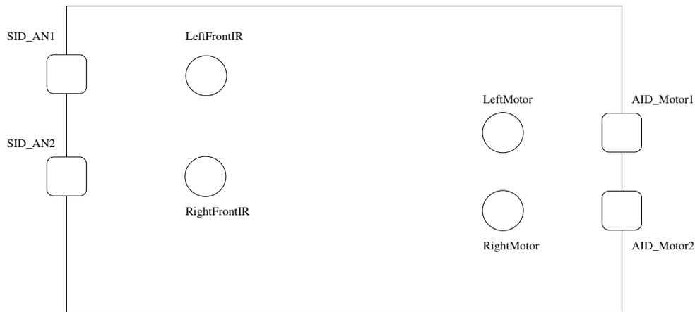
**Figure 2.8:** The construction of a PDL network. The program has serial ports SID\_AN1 and SID\_AN2 for analogue sensory input. Ports AID\_Motor1 and AID\_Motor2 are serial ports for the motors. The network consists of the quantities LeftFrontIR, RightFrontIR, LeftMotor and RightMotor.
