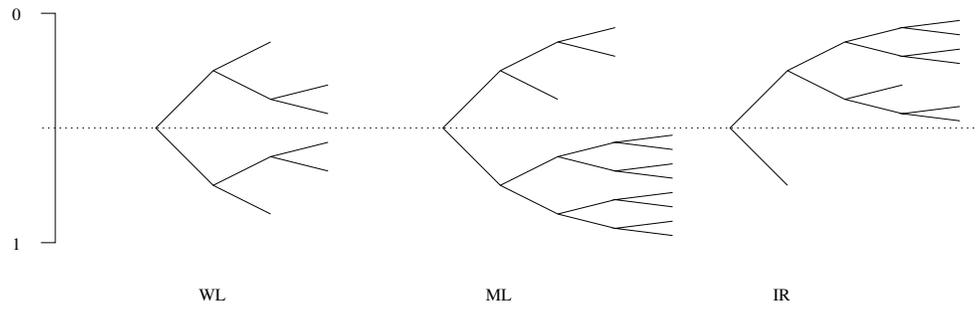
**Figure 3.9:** Categories represented as binary trees. Every sensory channel (like WL, ML and IR) is associated with a category tree. The root node of the tree is sensitive to whole range of the sensory channel. The tree is incrementally constructed during the evolution of discrimination games. Every time the discrimination game fails, two new nodes may be constructed by splitting one node.
