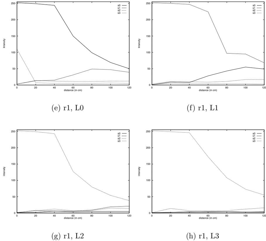
**Figure 2.5:** The characteristics of the calibrated light sensors as empirically measured for the experimental set-up when exposed to light sources  $L0 - L3$ . Plots (a) - (d) show the of robot r0 and plots (e) - (h) show them for r1. The distances are measured from the front of the robots to the boxes. Actual distances from source to sensor are  $12\text{cm}$  further.
