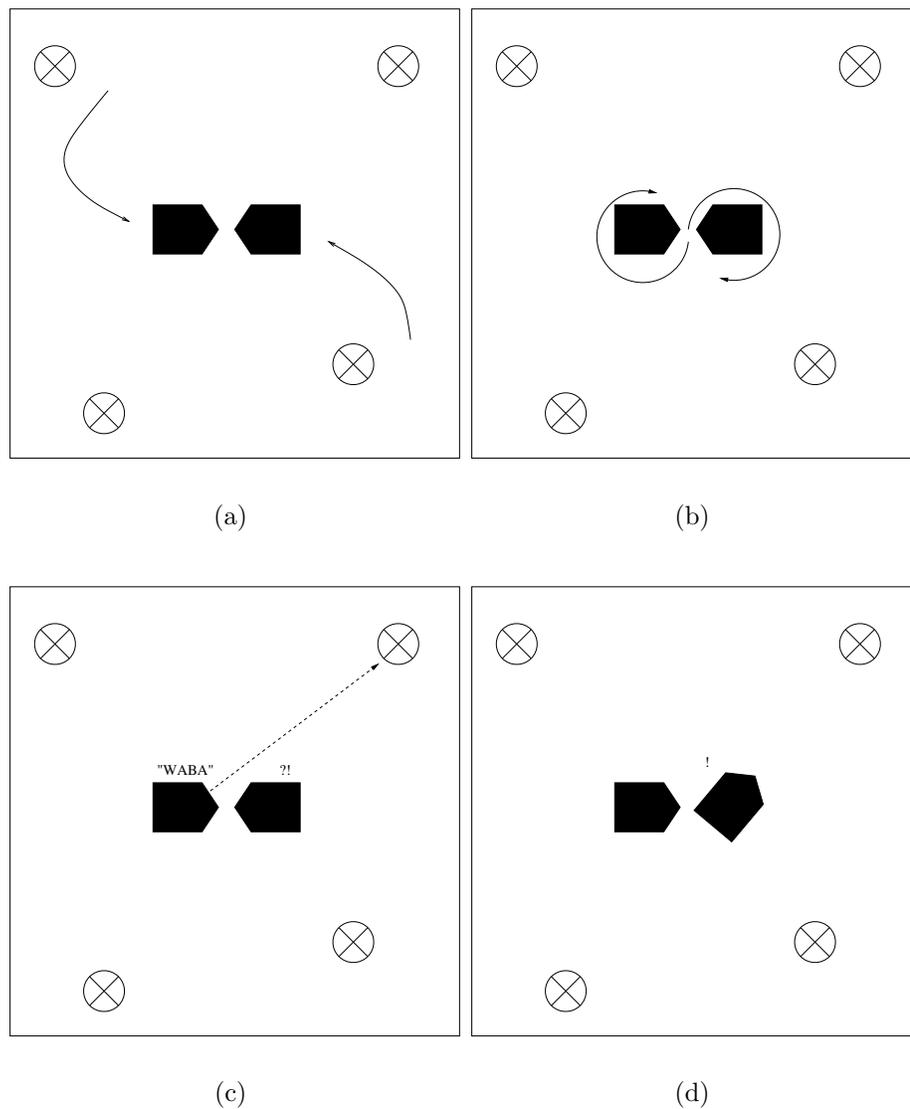
**Figure 3.1:** A temporal overview of the language game scenario. (a) The robots get together aligned and align. (b) The robots rotate in order to sense their surroundings. (c) The speaker produces an utterance and the hearer tries to understand the speaker. (d) When the hearer ‘thinks’ it understood the speaker, feedback is established and the robots’ memories are adapted.
