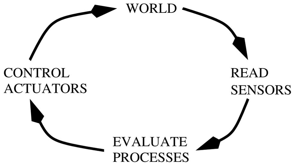
**Figure 2.7:** The way that PDL interacts with the world via a robot. Every  $\frac{1}{40}s$  PDL is going through a cycle as shown in the figure.
