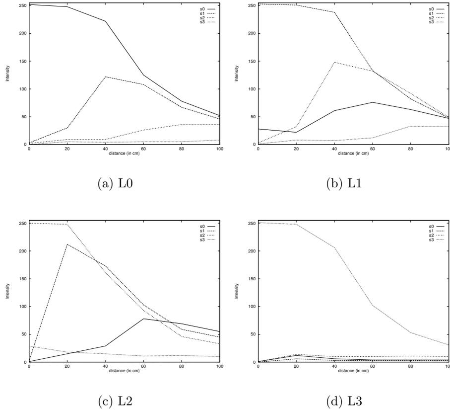
**Figure 5.3:** The characteristics of sensors s0, s1, s2 and s3 of robot r0 while looking at light sources (a) L0, (b) L1, (c) L2 and (d) L3. The light sources are placed at heights with a difference of 1.9 cm in between. Note that the characteristics of L3 may be inaccurate since the characteristics is quite different from all other characteristics.
