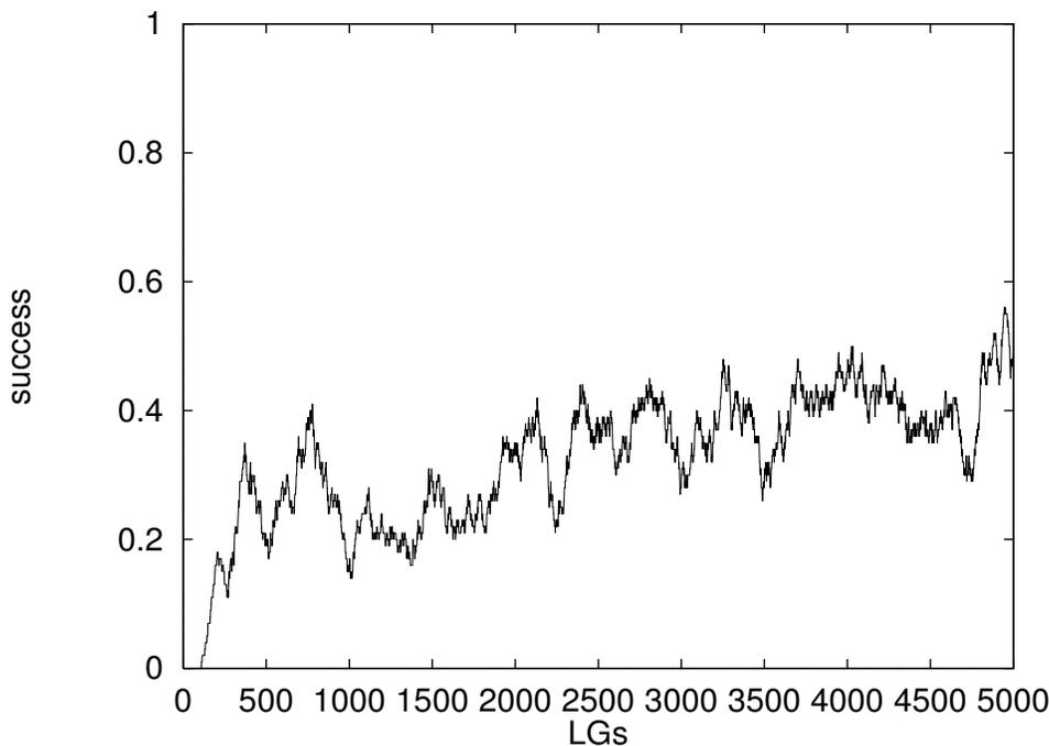
**Figure 4.3:** The communicative success of one run. The evolution shows a fast increase towards 30 %, after which it slowly grows to 50 % at the end. The evolution further shows a lot of fluctuations. Apparently the robots learn to communicate with ups and downs. A lot of these fluctuations are caused by polysemy and synonymy in the system as will become clear hereafter.
